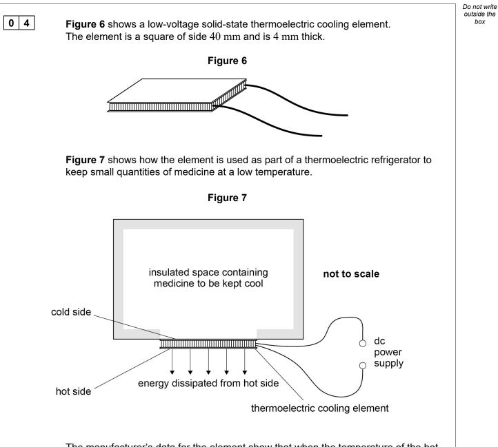
The manufacturer's data for the element show that when the temperature of the hot side is  $35 \,^{\circ}$ C and the temperature of the cold side is  $5 \,^{\circ}$ C:
